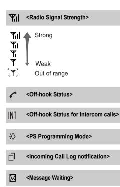
When you receive a message while in standby mode, the PS will alert you by vibrating or ringing, depending on the current setting of the Ringer Volume.
