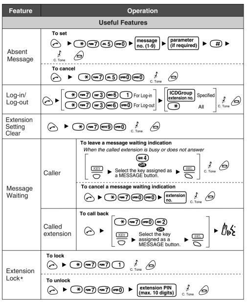
\* If an extension PIN has not been set for the PS, the extension cannot be locked. (Refer to the Business Telephone System User Manual)
