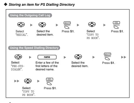
• When storing an outside phone number, the line access number will be stored automatically. The line access number must be identical to the PS's "TRUNK ACCESS CD" setting (SYSTEM SETTING). (See page 40.)
