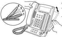
The tilt angle of the operation board can be adjusted to one of four angles.
