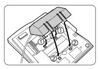
Pull down the handset hook until it locks, so the tab holds the handset.
