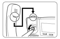
To prevent damage to the telephone, be sure to unplug the extension line before you set up or remove the USB Module or the Add-on Key Module.
